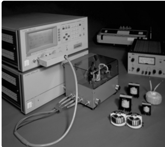
High current bias for inductor testing under load conditions
